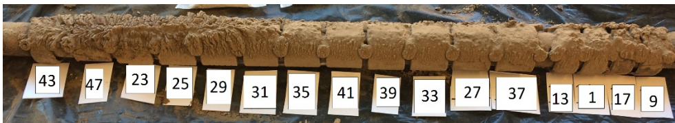
Figur 10. Korrosionssonden efter exponering med proverna fortfarande fastmonterade Figure 10. The corrosion probe after exposure with the specimens still mounted
