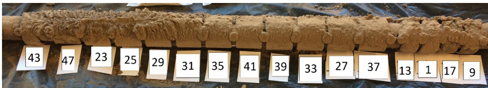
Figure Summary-4. The corrosion probe after exposure with the specimens still mounted
