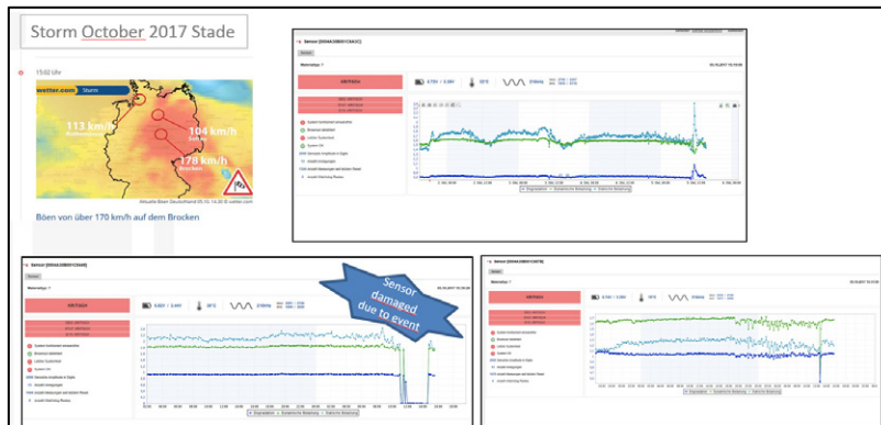
Figure A5. During a storm a tree fell on a pipe which was detected by the lamb wave sensor technology.
