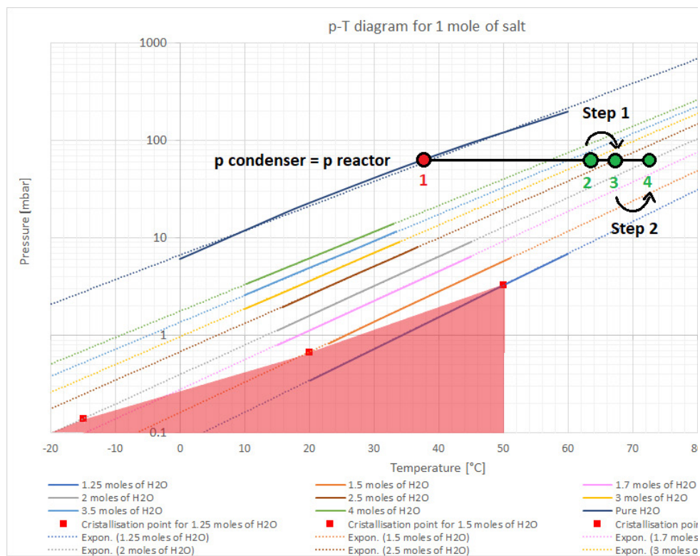
Figure 8 Steps of the charge process on the p-T diagram
