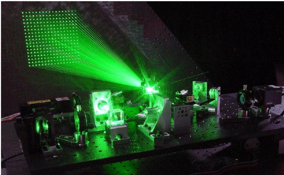
Figure 11. 256-beam WF-LDV at laboratory [13].
