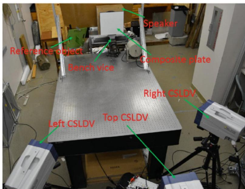
Figure 14. Setup of the 3D-CSLDV system [15] .
