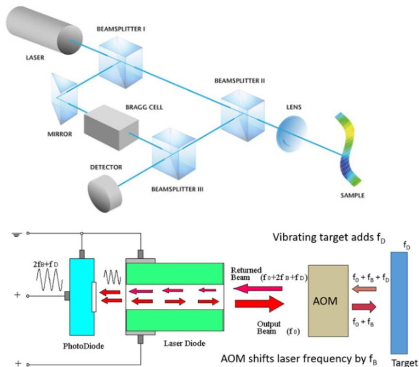
Figure 7. Heterodyne self-mixing interference system schematic (by Polytech and OMS).
