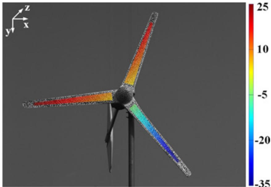
Figure 17. Full-field displacement distribution of the wind turbine blades (z direction, units in cm). [2]
