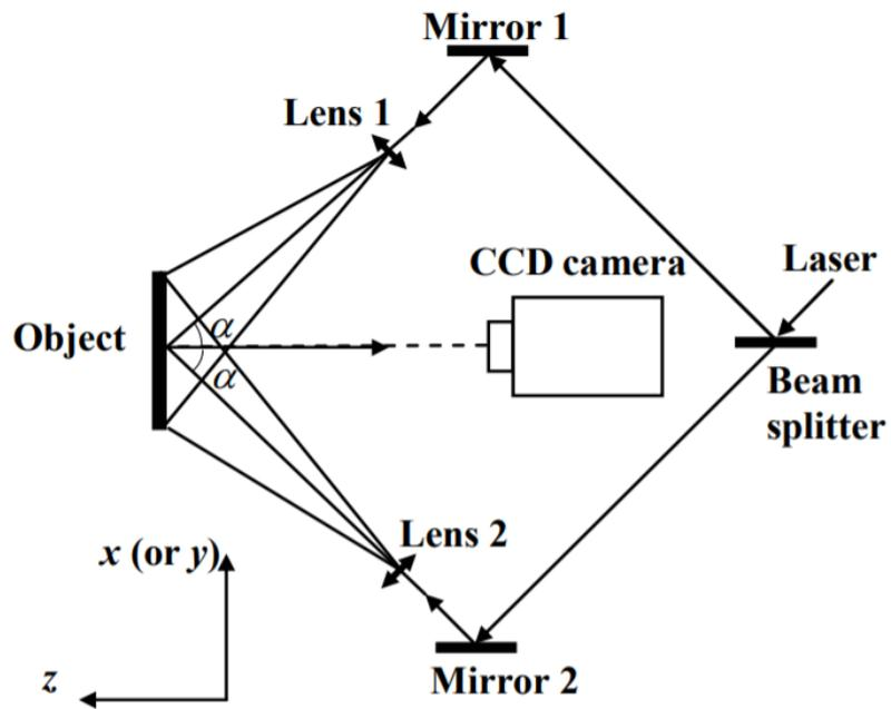
Figure 16. Schematic of in-plane ESPI setup [18].
