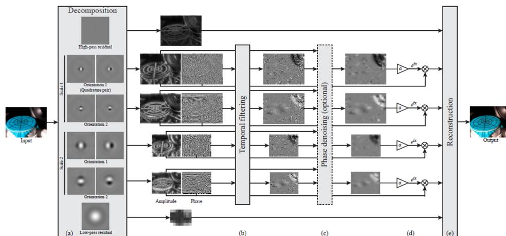
**Figure 5. Phase-Based improved Motion magnification workflow: (a) 2D complex steerable pyramid filters decompose the video into amplitude and phase at different scales, (b) the decomposed phases are band pass filtered in frequency, (c) amplitude-weighted smoothing is applied, (d) the band passed phases are amplified or attenuated, and (e) the video is reconstructed [8]**
