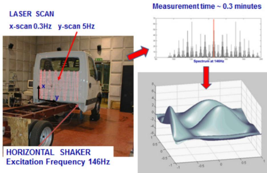
Figure 13. Continuous-scan laser Doppler vibrometry. Vehicle cab scan pattern (left), velocity spectrum (top right) and reconstructed ODS (bottom right) [10].
