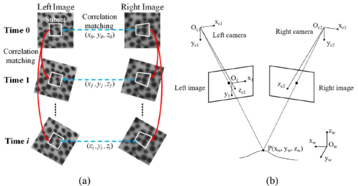
**Figure 1. A schematic diagram of the principle of 3D-DIC. (a) Correlation matching procedure, (b) 3D reconstruction procedure involving two cameras [2].**
