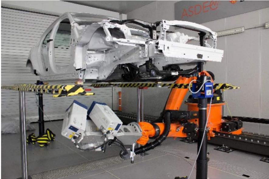
Figure 8. 3D SLDV on a whole vehicle body: instruments mounted on a robot arm [10].
