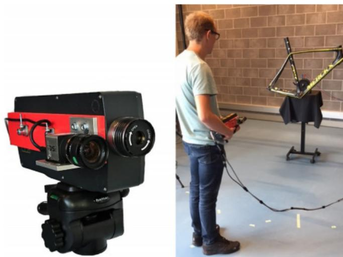
Figure 22. Handheld LDV experiment: Polytec IVS200 attached with IDC  $\mu$ Eye camera (Left). Handheld LDV measurement of bike frame excited with shaker (Right). [29]
