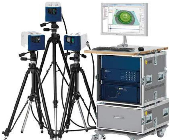
Figure 9. Setup of the 3D SLDV system (Polytech)
