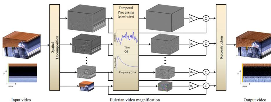
**Figure 4. Overview of the Eulerian video magnification framework: Laplacian pyramid, Intensity band pass filtering, Amplifications of filtered intensity signal and video reconstruction. [6]**
