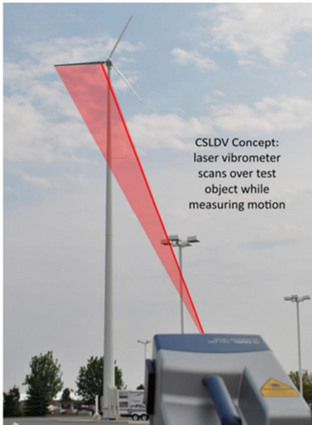
Figure 18. Wind turbine blade deflection measurement with CSLDV [23].
