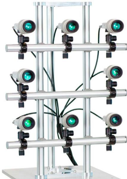
**Figure 12. 8-channel optical setup of Polytec Multipoint Vibrometer.**
