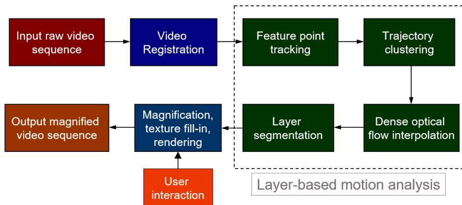
**Figure 2. Layer-based motion magnification pipeline.**
