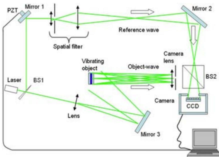
Figure 15. Diagram of holographic interferometry measurement system setup [16].
