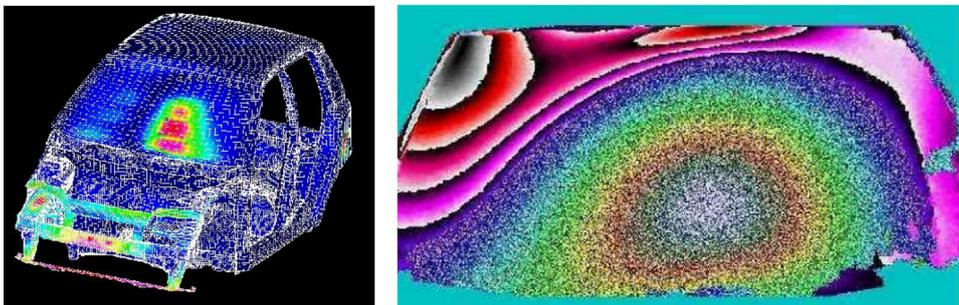
Figure 19. Operational deflection shapes of wind screen at 100Hz frequency: FE-calculated (left), ESPI (right) [25].
