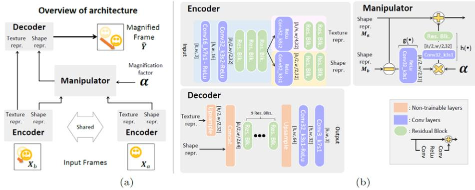
**Figure 6. Deep Convolutional Neural Network Architecture consist of three parts: Encoder, Manipulator and Decoder. [9]**
