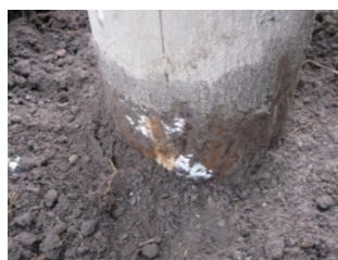
Ecopole 7491. Mycel under markbandet
