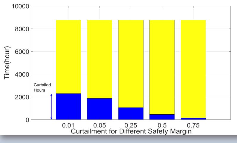
Hours with curtailment as a function of the acceptable probability of overload
