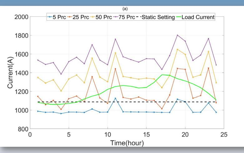
Static rating (dashed line) and four different probabilistic dynamic ratings (solid curves) together with line current (green) for a **winter**
