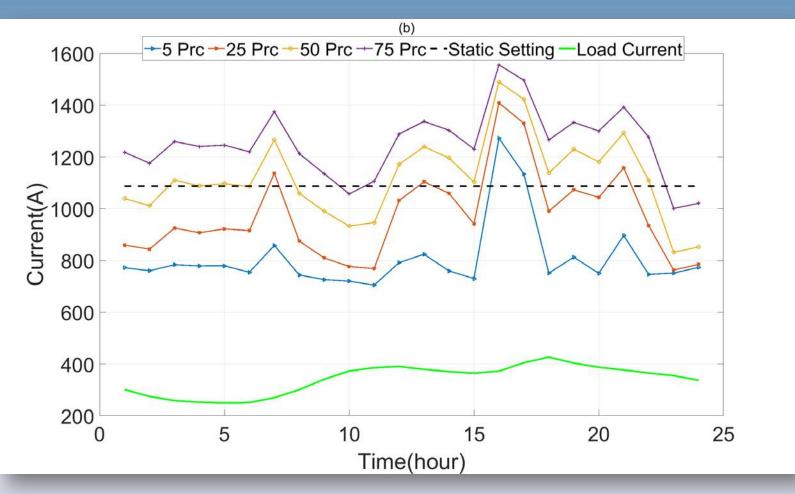
Static rating (dashed line) and four different probabilistic dynamic ratings (solid curves) together with line current (green) for a **summer**
