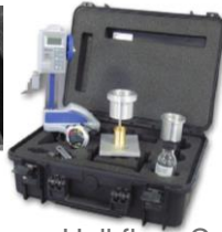
Hall flow, Carney flow and apparent density
