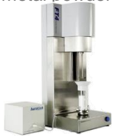
Semi-automatized tapped density method producing compaction curve as a function of number of taps for a SLM metal powder
