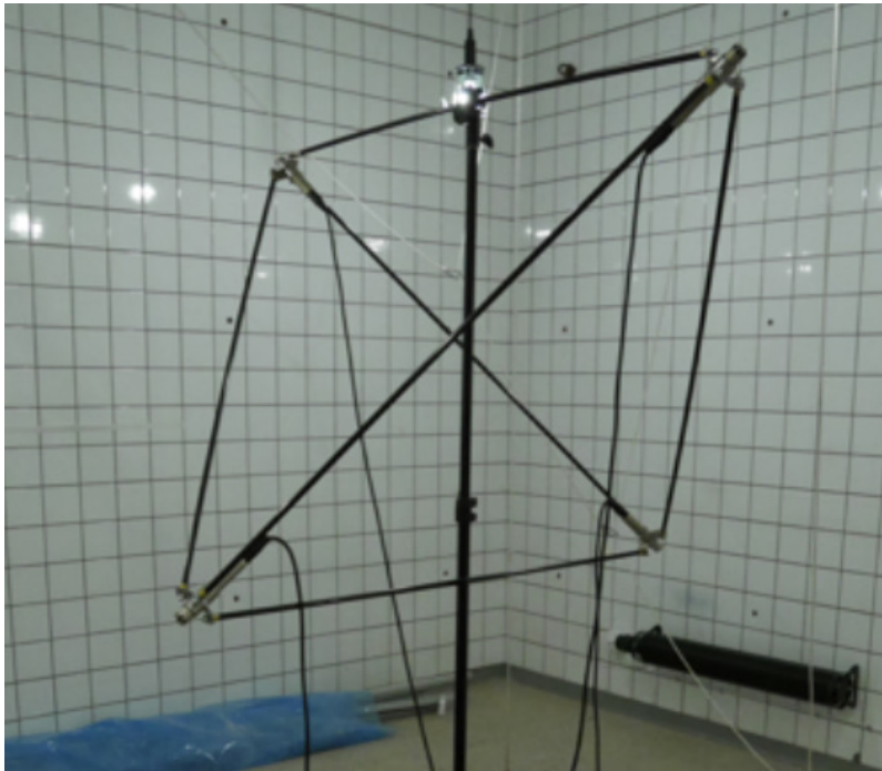
Figure 2: Arrangement of the tetrahedral array in the reverberant chamber.
