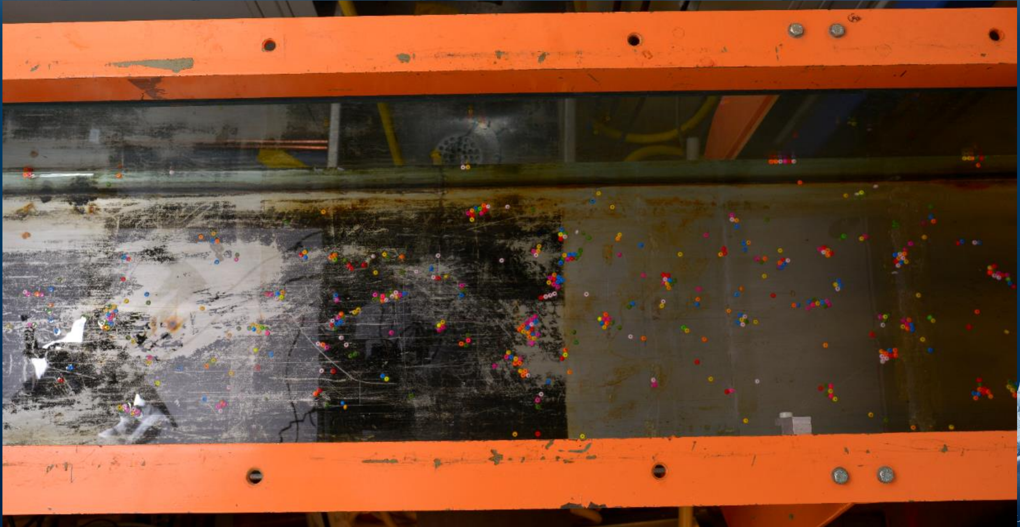
Image of channel flow with seeding particles
