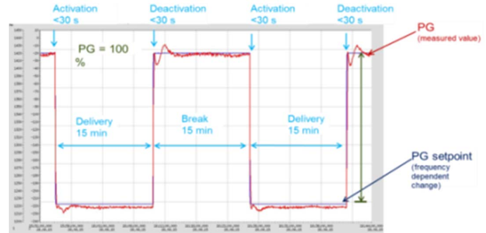
World record for FCR with NPPs: Successful qualification test of downwards 200 MWel
