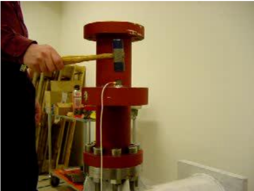
REGULAR PIPE WITH NATURAL LOW DAMPING
