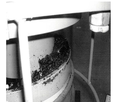
Viscodamper with cracked fluid
