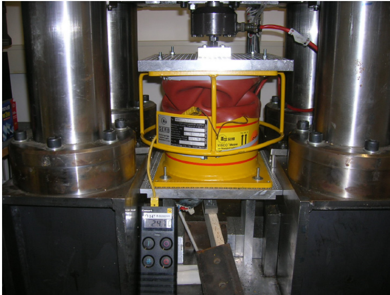
Figure 81: Test rig verification of a VES-5/V40/H40 GERB damper. Damping resistant and dynamic stiffness are measured at different temperature during a stepped sine test. Test rig belongs to Efterklang® (part of AFRY)
