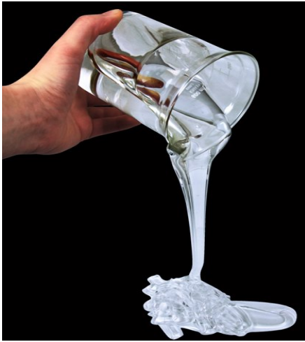
Figure 15: The silicone/bitumen can be extremely thick, and viscosity depends on temperature. In picture silicone folds back and forth on itself almost like a ribbon. This is an example of high viscosity.
