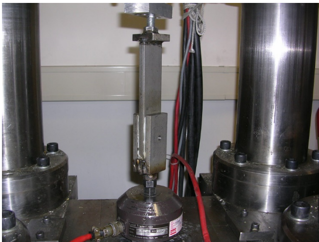
Figure 75: Damper link installed in a servo-hydraulic test rig which belongs to Efterklang®. Test rig conforms to ISO10846-2. Picture shows initial damper link status for 0 cycles.
