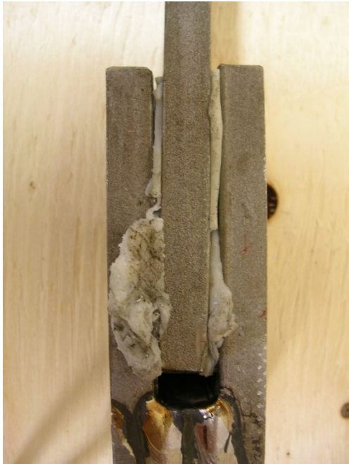
Figure 78: Broken and repaired damper link. The viscoelastic polymer is self-adhesive.
