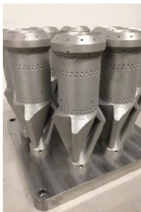
Siemens additive manufactured burner used in SGT-600, SGT-700 as well as in SGT-800. Also available for retrofit in existing units.
