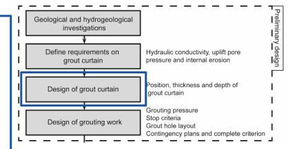
Design the grout curtain as a structural component of the dam foundation, instead of a foundation treatment under the dam.
