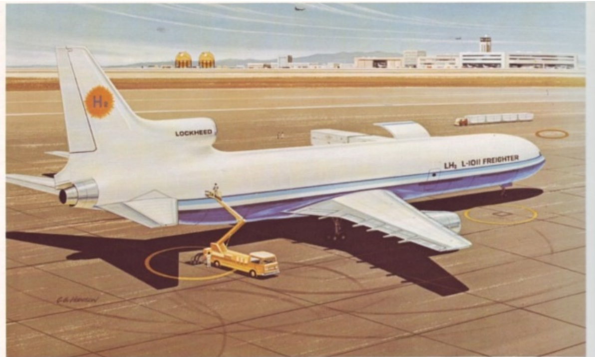
A Candidate Liquid-Hydrogen (LH 2 ) Fueled Prototype Freighter Aircraft—An L-1011-500 transport, stretched nearly 40 feet to provide room for LH 2 tanks fore and aft of a cargo compartment, has been suggested as a candidate for a demonstration flight program to ascertain the practicability of using LH 2 as fuel for future transport aircraft.
