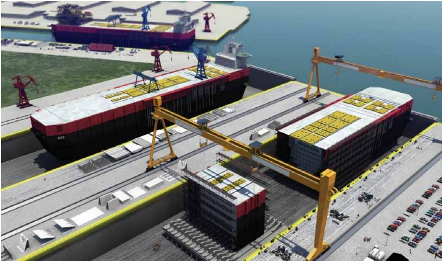
Modular blocks are added to an FPSO under construction in a dry dock.
