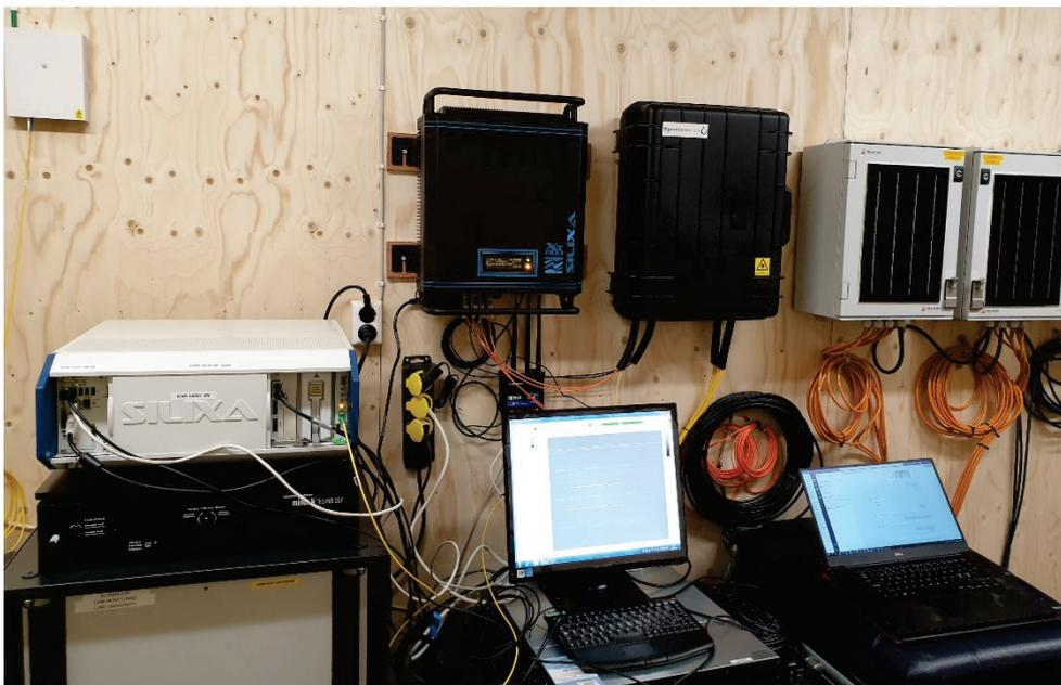
Figure 4 Monitoring unit for DAS and DTS, inside the monitoring container.
