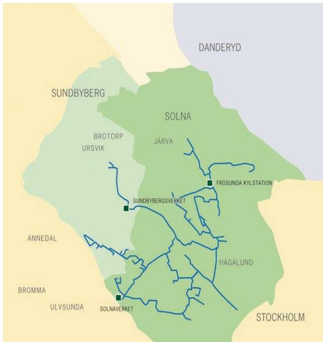
**Figure 2. Norrenergi AB's DC system today, with the three cold production plants Sundbybergsverket, Frösundaverket and Solnaverket (also including the existing CS)**
