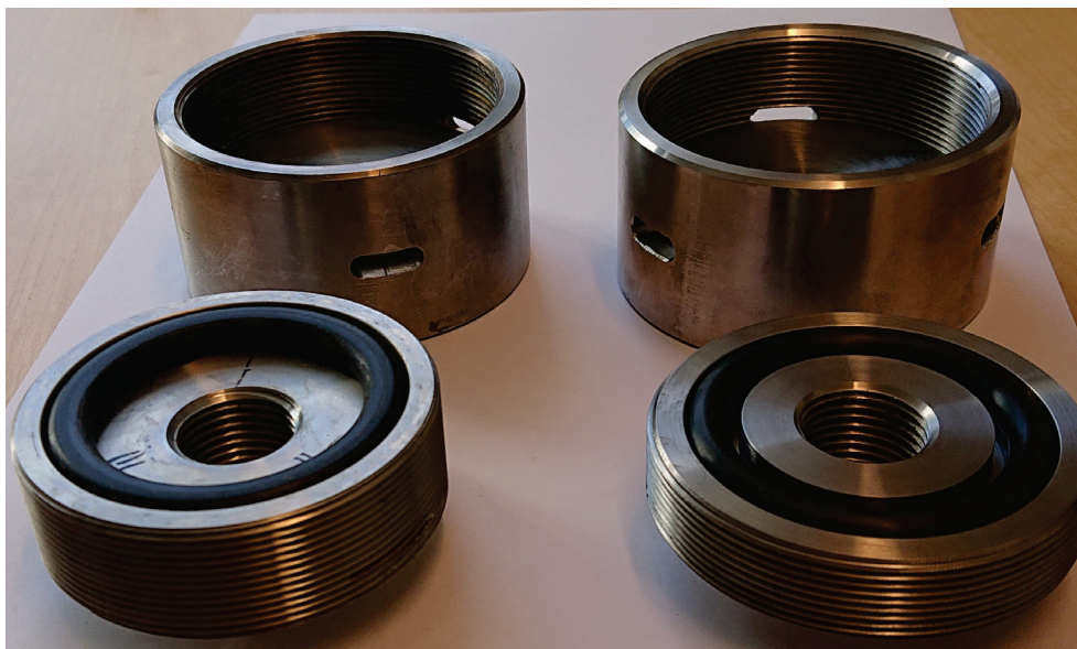
Figure 4. O-ring test rigs. Left: old test rig from COMRADE. Right: new test rig re-designed for SAMPO.
