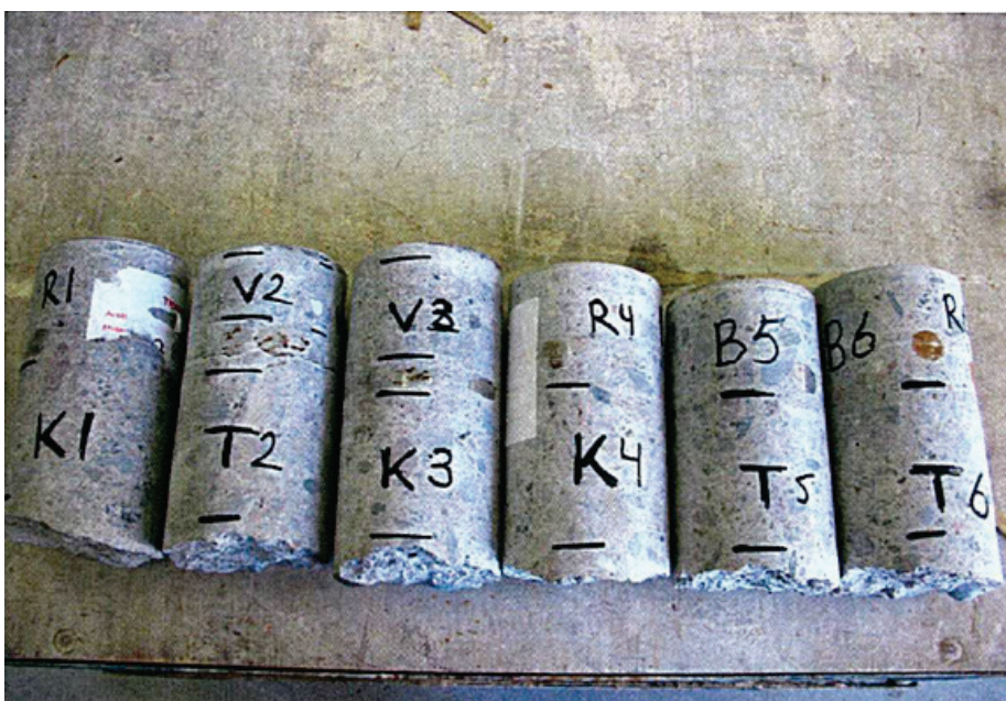
Figure 3-1. Concrete cores extracted from a concrete structure in Forsmark NPP.
