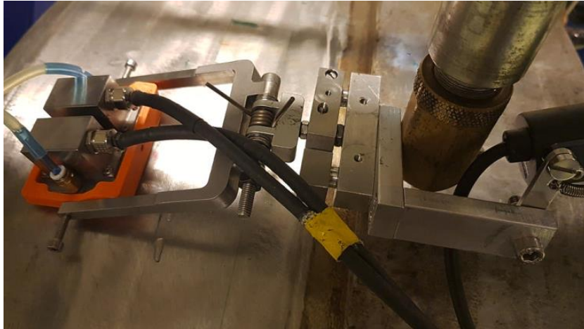
Figure 12. Scan setup for dissimilar weld mock-up. Adapted from Virkkunen et al. [32]. Observe the water-feed to the transducers to the left in the figure. Licensed under CC BY 4.0.
