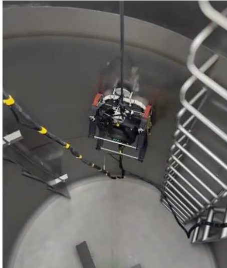
Figure 22. HausBots HB2 deploying UT probe inside a stainless-steel tank. Image courtesy of HausBots Ltd.
