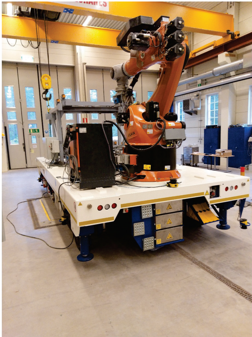
Figure 6 The mobile robotic vehicle is equipped with lots of sensors which also creates the safety feature of the robots work cell.
