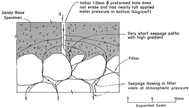
**Figure 5.3** Condition at end of successful test on silty and clayey sands with low fine contents (Sherard & Dunnigan, 1989).
