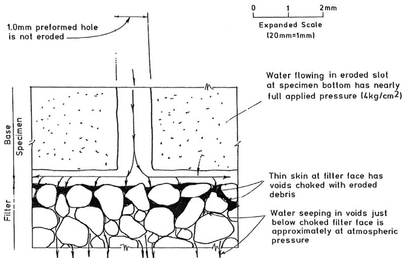
**Figure 5.2** Condition at end of successful test on fine silts and clays (Sherard & Dunnigan, 1989).
