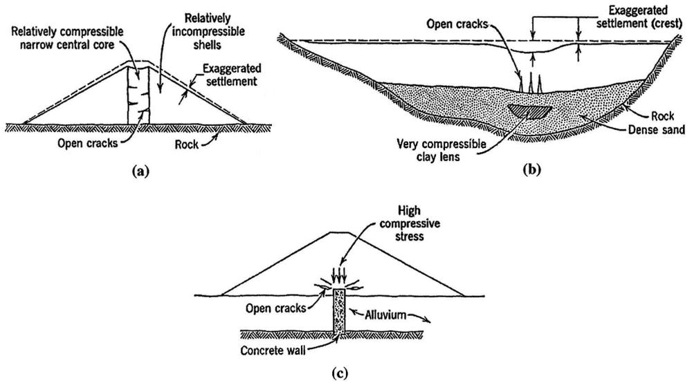
**Figure 3.8** Typical internal differential settlement cracks in embankments (Sherard *et al.*, 1963).
