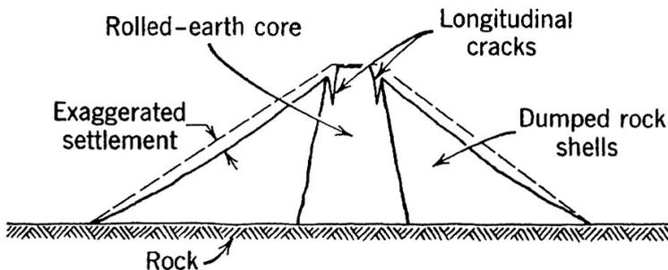
**Figure 3.6** Longitudinal differential settlement cracks between embankment zones (Sherard *et al.*, 1963).
