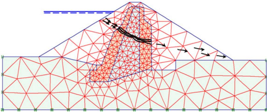
**Figure 8.1** Numerical modelling of internal erosion.
