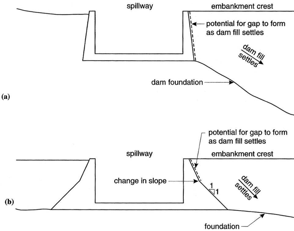
**Figure 3.9** Situations where a crack might form between the dam fill and the spillway wall: (a) steep foundation adjacent to spillway wall; (b) change in slope of the retaining wall (Fell *et al.*, 2005).
