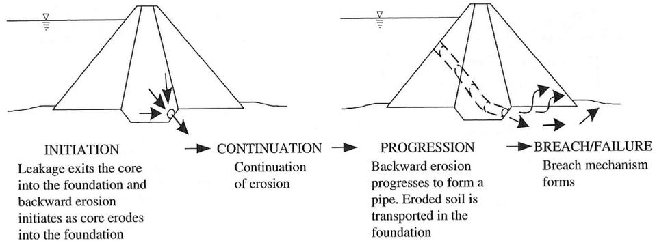
**Figure 3.3** Conceptual model for development of failure by piping from the embankment into the foundation (Foster, 1999).
