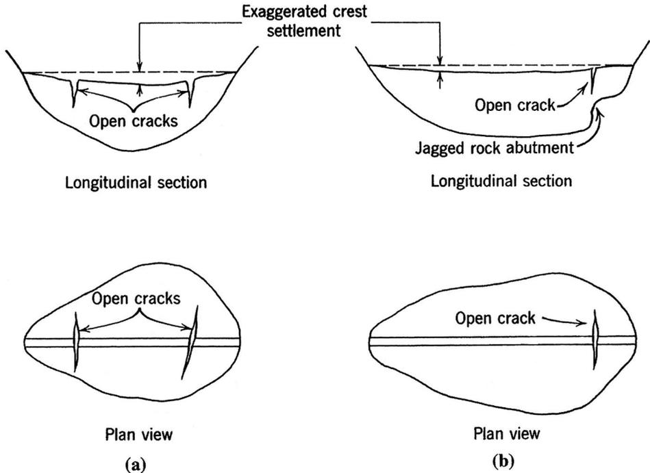
**Figure 3.5** Ordinary transverse differential settlement cracks.
