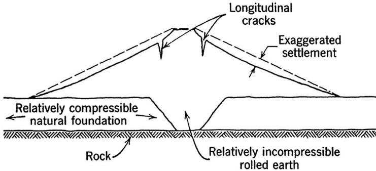
**Figure 3.7** Longitudinal differential settlement cracks over foundation discontinuities (Sherard *et al.*, 1963).
