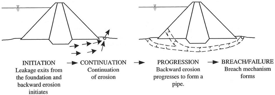
**Figure 3.2** Conceptual model for development of failure by piping in the foundation (Foster, 1999).
