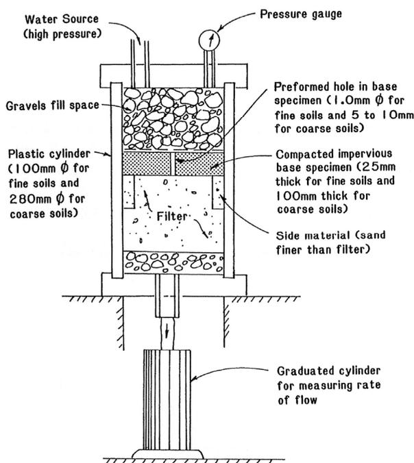
**Figure 5.1** The no erosion filter test (Sherard & Dunnigan, 1989).
