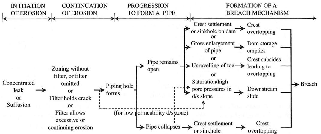
**Figure 3.4** Failure path diagram for failure by piping through the embankment (Foster, 1999).
