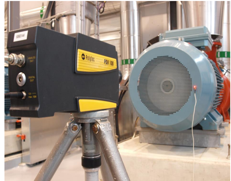
Laser Doppler Vibrometer, LDV Accelerometer ICP
