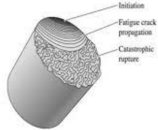
Appearance of typical fatigue fracture surface
