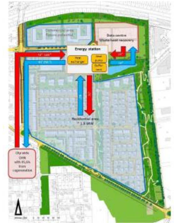
Figure 82. Excess heat recovery from data centre in Braunschweig/Germany.
