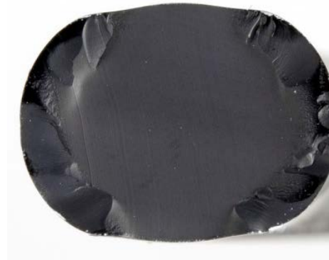
Cut cross-section of HNBR O-ring aged for 100 days at 150°C
