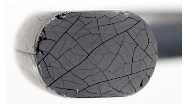
HNBR O-ring after 1 year at 150°C
