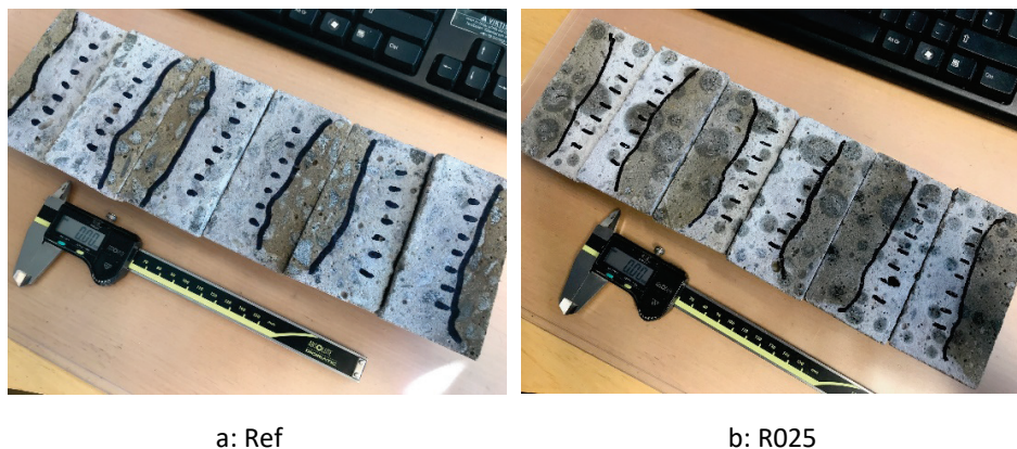
Figure 4.5 – Cross-sections of concrete after compression test.
