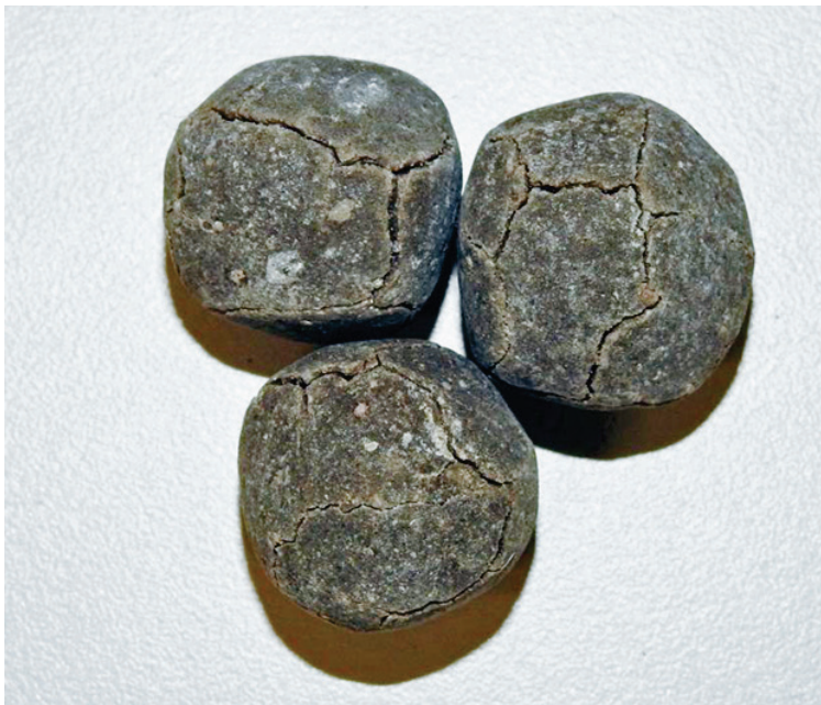
Figure 3.2 – Cracking probably due to the metallic aluminium (release H_2 gas under the alkaline environment).
