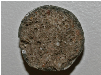
Figure 4.4 – Air bubbles inside the stone balls made from R025 GBA.
