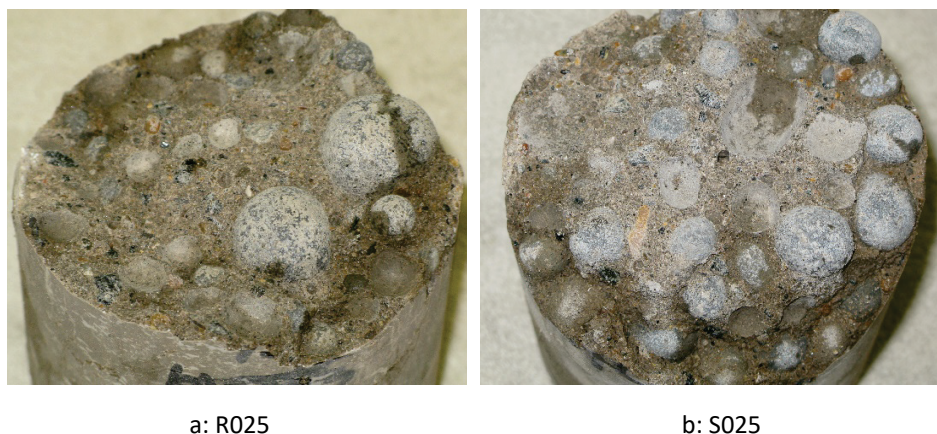
Figure 4.5 – Cross-sections of concrete after compression test.
