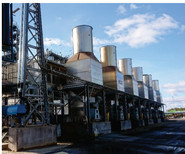
Figure 4. Belt dryer for sawdust (left) and storage silo (right) at the Värö mill.
