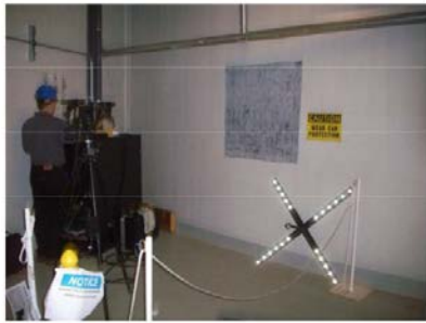
DIC application during a containment pressure test: (a) DIC cameras and inspection location; and (b) principal strain at 0.24 MPa showing strain concentrations – a sign of hairline cracks on the concrete surface
