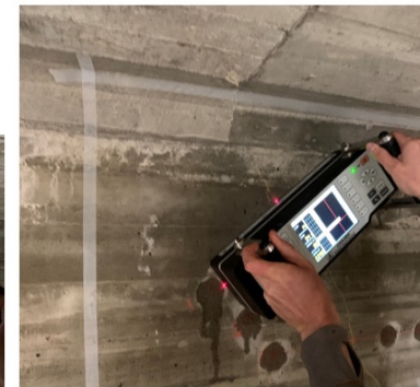
Damage detection along cables (grouting defects, corrosion, etc.)
