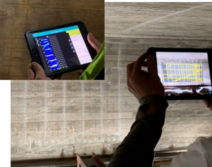
Detect steel tendons in pre/post tensioned RC bridges
