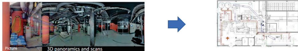
Figure 14 Visual positioning based on 3D scans and panoramic photos
