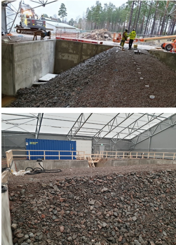
Figure 1 Pictures of the crest and downstream face and upstream face of the test dam before filling.
