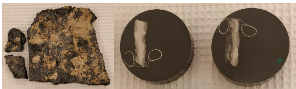
Figure 25 Sample from the cyclone vortex finder, retrieved in Mälarenergi P6 boiler. The sample was cut into two cross sections that were mounted in conductive bakelite for further examination.
