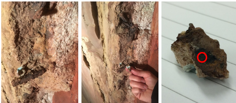
Figure 15 Retrieved studding from boiler Händelö P14. The encircled area corresponds to the chemical analysis shown in Table 3.
