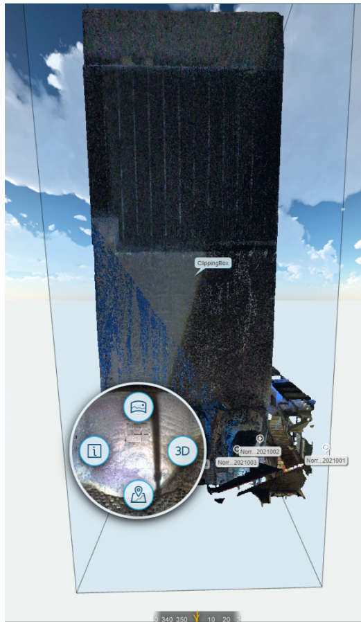
Figure 56 Use of the 3D scan cloud to orient and check detailed areas in various views such as panoramic.
