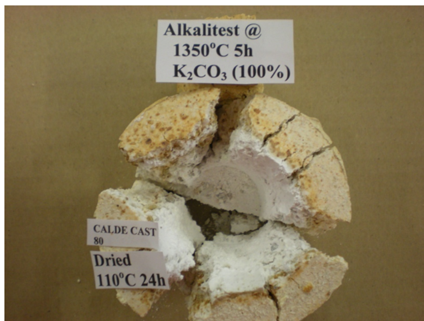
Figure 73 Photos of a high-quality refractory without the proper alkali resistance needed.
