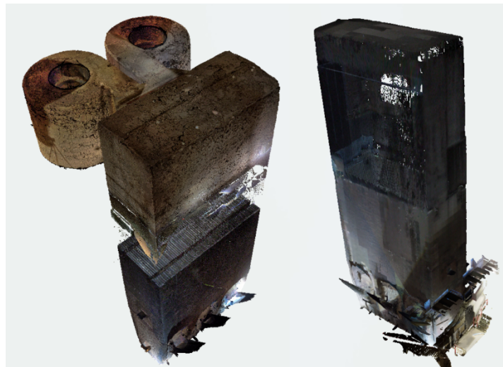
Figure 54 3D cloud image from multiple scan positions giving a 360 degree image fully measurable.
