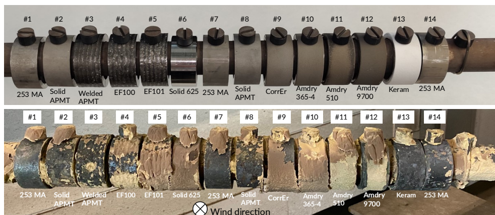
Figure 34 Metallic rings before and after exposure. The rings were fastened to the probe with Kanthal® APMT™ bolts to prevent potential shift during exposure. The bolt corresponding to one of the specimens was lost during the probe installation process and consequently the specimen was rotated approximately 90° with respect to the others. The wind direction is shown in the bottom picture.
