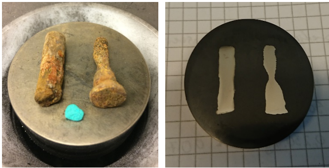
Figure 28 Studdings retrieved from Mälarenergi P6 boiler system. The right image shows the studdings mounted in conductive bakelite and ground to reveal their cross sections.
