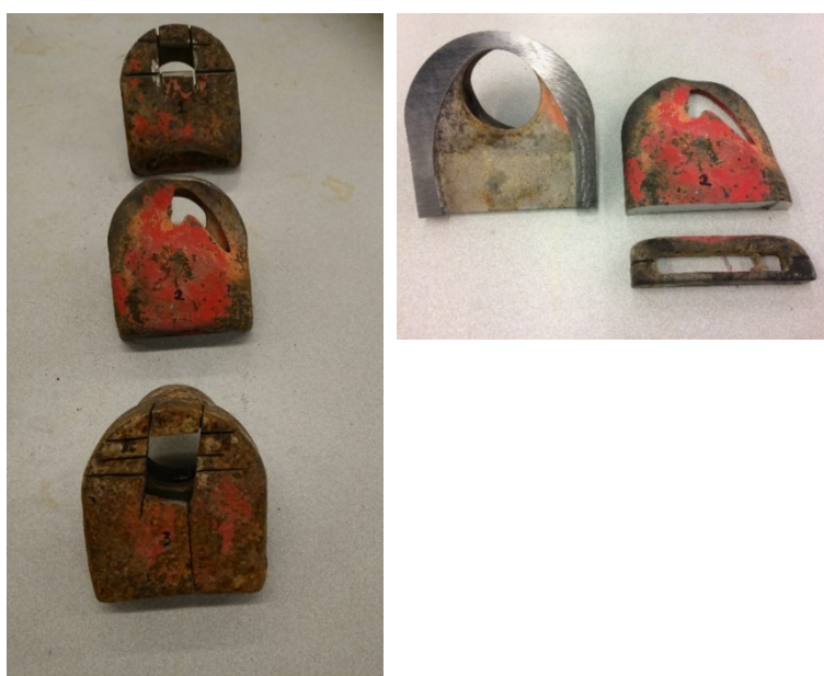
Figure 27 Primary air nozzle retrieved from Mälarenergi P6 boiler system. The nozzle exhibited evidence of erosive wear.
