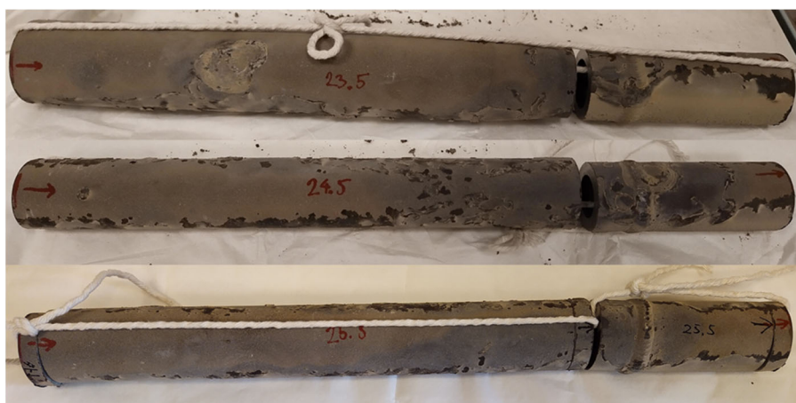
Figure 18 Appearance of the removed tubes and cutting of sections. Tube 23.5: 304HCu; Tube 24.5: 347HFG; Tube 25.5: 347H; Tube 25.5 right: 310HCbN
