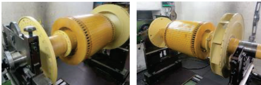
Figure 64: Large vertical motor with extra balancing plane reachable from the outside by a lid in the motor house.
