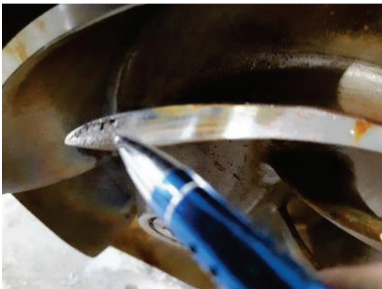
Figure 20: Pump impeller with pitting damage at the vanes
