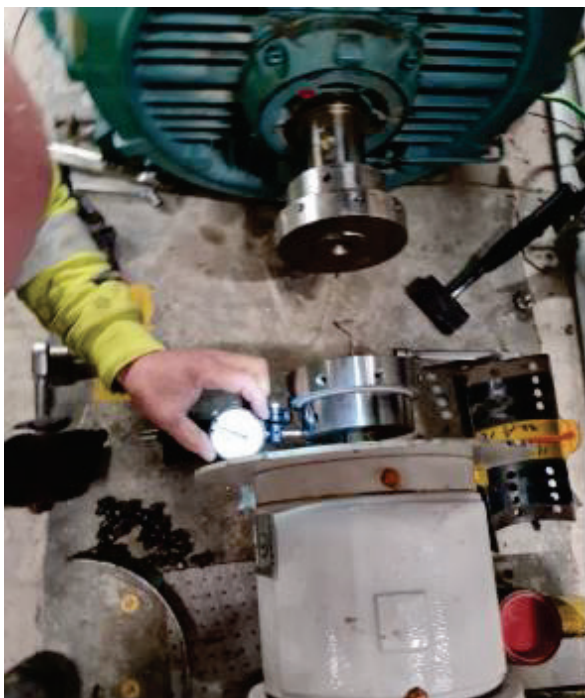
Figure 47: Checking coupling runout at the pump side with an indicator clock
