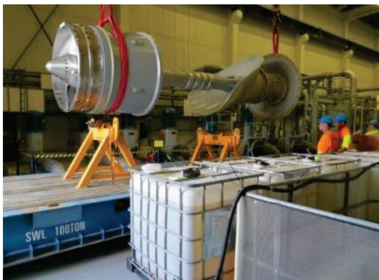
Figure 8: Main Coolant sea water pump of centrifugal type with axial-flow
