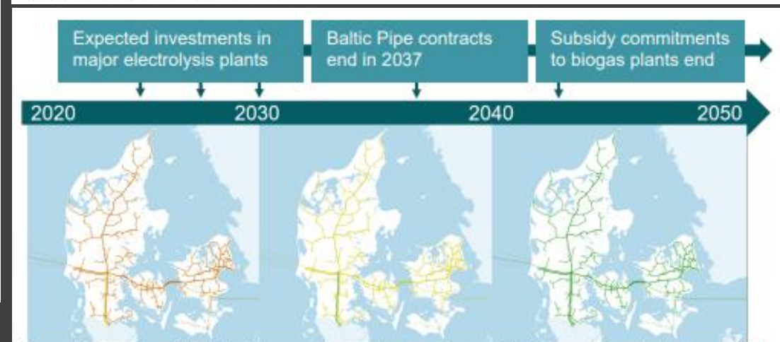
Figure 11. Overview of the Danish gas system and conversion possibilities over time. Red: No possibility for conversion, yellow: Some possibility for conversion, green: Good possibilities for conversion. Note the pipeline in South Jutland which can potentially be converted to hydrogen export in the medium term. Source: The Danish Energy Agency
