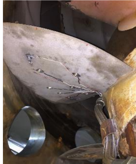
Pressure and strain measurements on a Kaplan prototype; Porjus U9 (A. Soltani, 2018)
