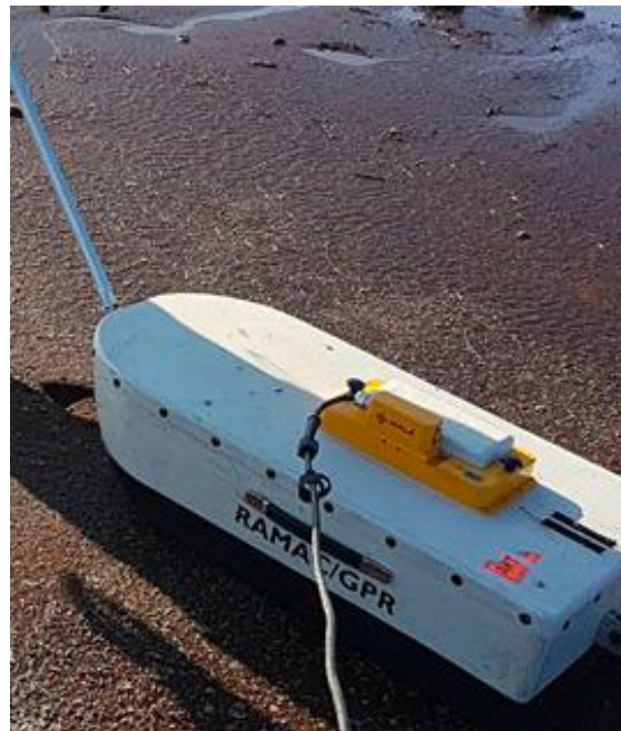
Figure 1. The 250 MHz Ramac/GPR antenna system used for measurements. Measurements are done continuously while dragging the antenna along surface profiles.
