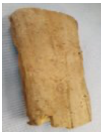
Figure 48. The hardened surface of Tremco sealing.
