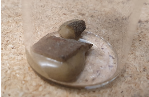
Figure 46. Tremco sealing after MC test at 90 °C.
