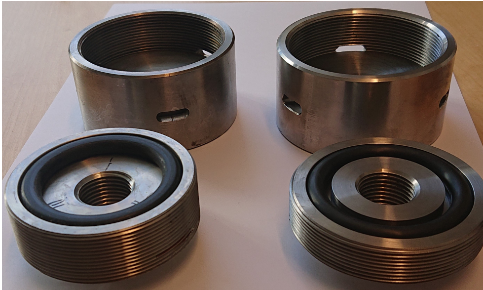
Figure 5. O-ring test rigs. Left: old test rig from COMRADE. Right: new test rig re-designed for SAMPO.
