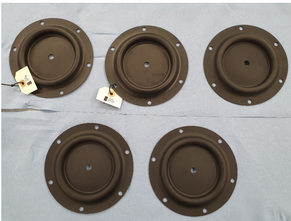
Figure 12. Photograph of new neoprene membranes from Ringhals NPP.
