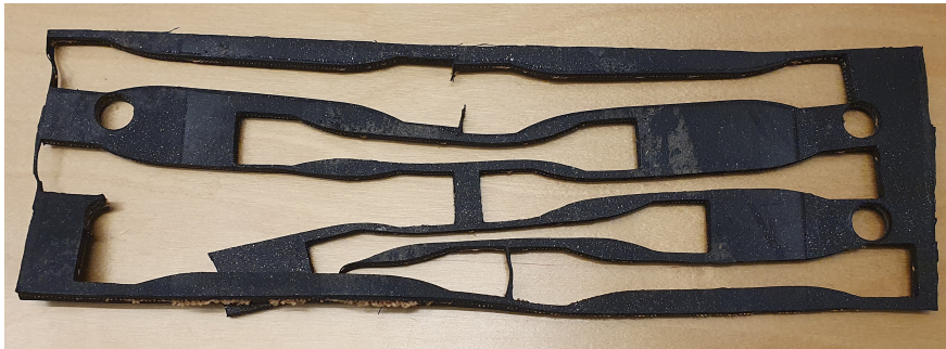
Figure 18. Photograph of joist seal received from TVO after sample preparation.
