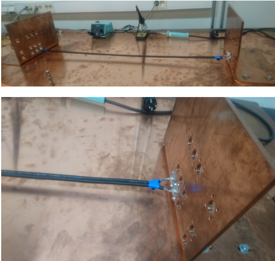
Figure 24. Cables mounted and taped to run parallel above the ground plane. The connectors are located on the outside of the copper angle brackets. Each of the wires is connected to the VNA in one end and a termination ( 50\ \Omega or short) is connected to the other end of that wire. If the wires are connected to the VNA at the same end, we call the measurement NEXT. If they are connected at opposite ends, we call it FEXT.
