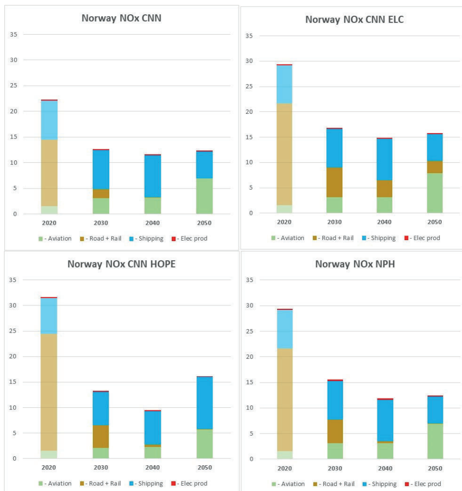
Figure 3. The modelled development of NOx emissions (in kton) for aviation, road transport including rail, and shipping as well as from electricity production for direct use in the transport sector in Norway in the assessed scenarios. For scenario descriptions see the text.
