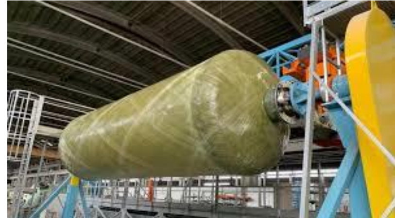
Pull winding process for composite
