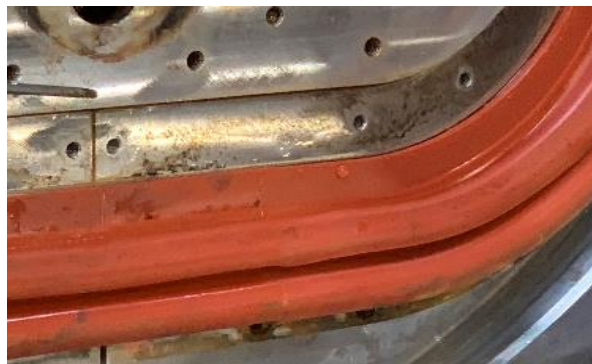
Qualification of the seal of Fla3 cofferdam
