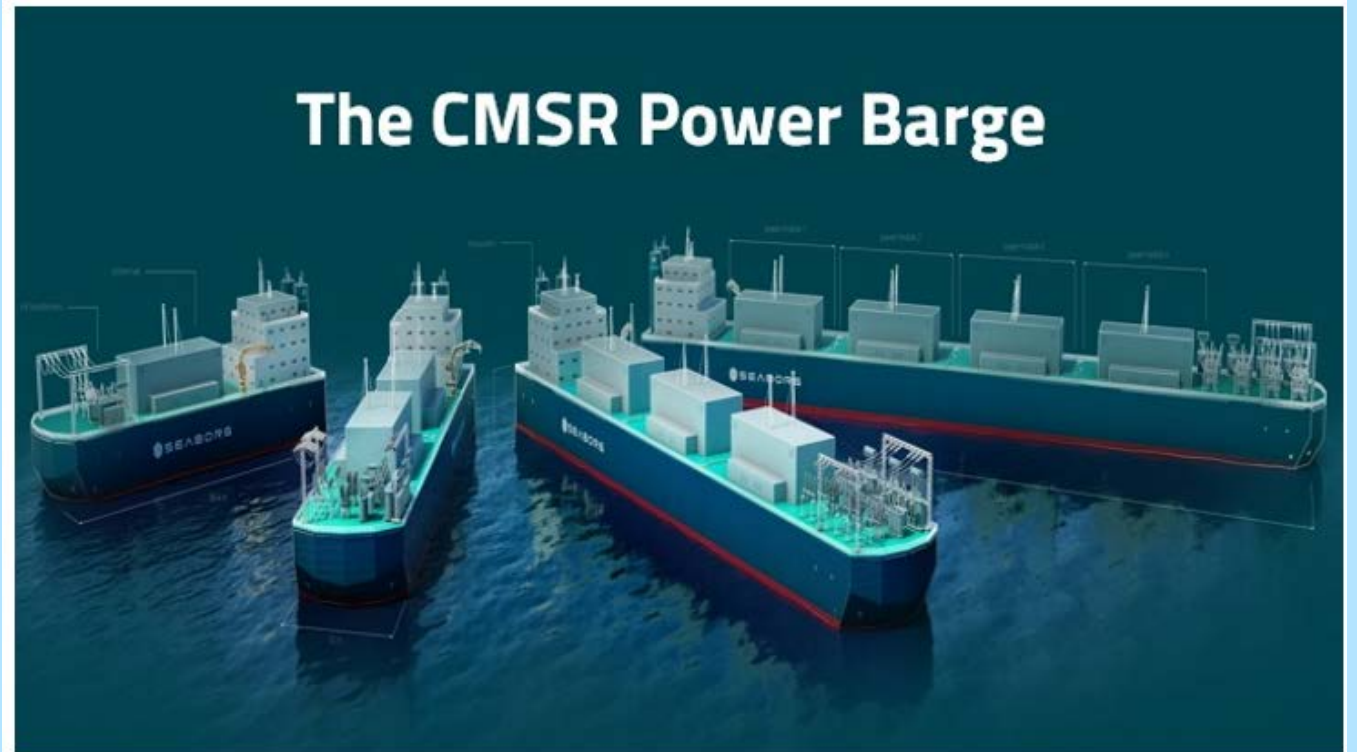
The Power Barges are modular and can produce from 200-800 MW of electricity (Image: SHI/Seaborg)
