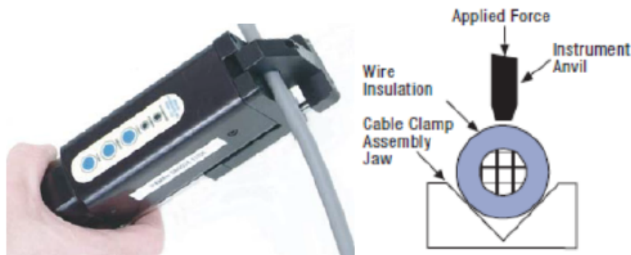
Figure 9. Indenter equipment and schematic measurement principle according to [Pirc 2016].
