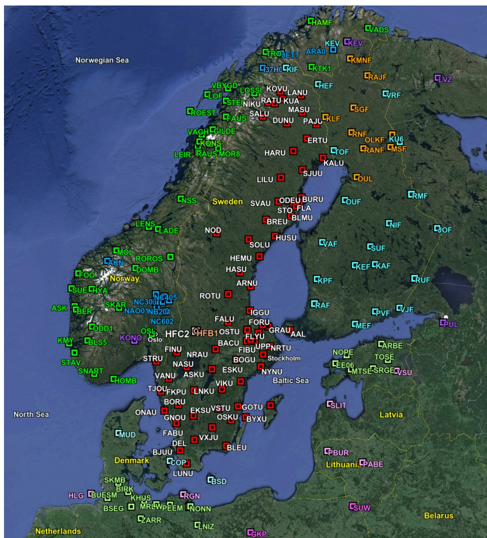
Figure 20 Seismic stations in permanent seismic networks in the Fennoscandian and nearby regions. The different colors of the stations indicate different network operators.
