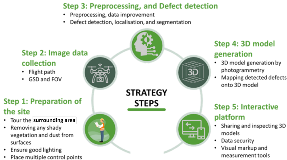
Figure 3-33 5-step strategy for remote inspection of concrete structures, using UAVs and computer vision.
