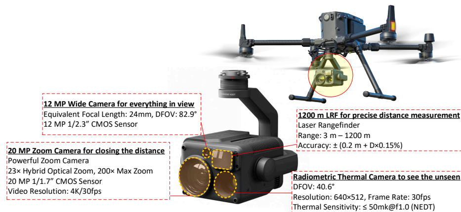
Figure 4-6 Matrice 300 RTK drone equipped with a H20T Quad-Sensor Solution unit.
