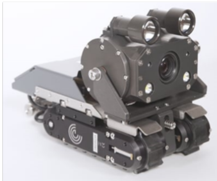
The Remotely Operated Robotic Crawler Solution for Confined Space Inspections in Nuclear Power Plants, designed by Eddyfi Technologies' robotic ( https://www.eddyfi.com/ )
