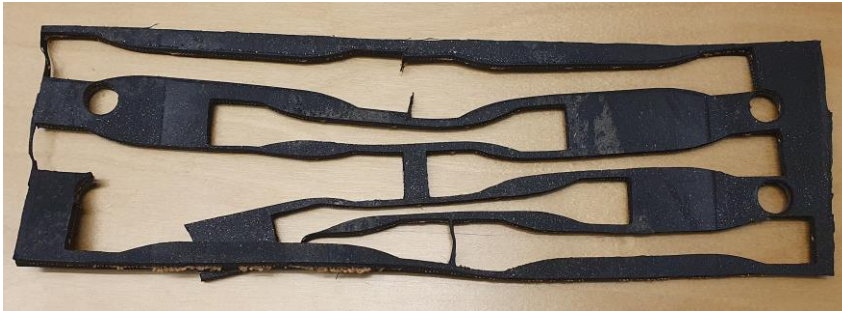
Figure 9. Photograph of joist seal received from TVO after sample preparation.
