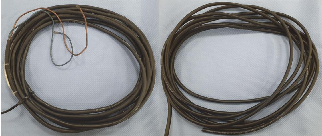
Figure 10. Photographs of CPE cables from Forsmark NPP (left) and reference cable (right).
