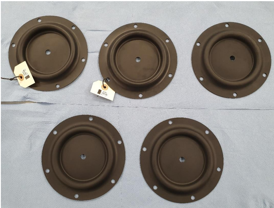
Figure 4. Photograph of new neoprene membranes from Ringhals NPP.
