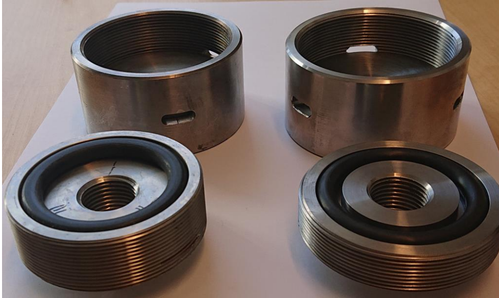
Figure 3. O-ring test rigs. Left: old test rig from COMRADE. Right: new test rig re-designed for SAMPO.
