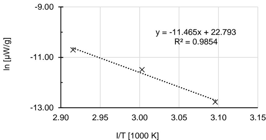
Figure 11. Arrhenius plot for commercial or grade 3 material with reinforcement.
