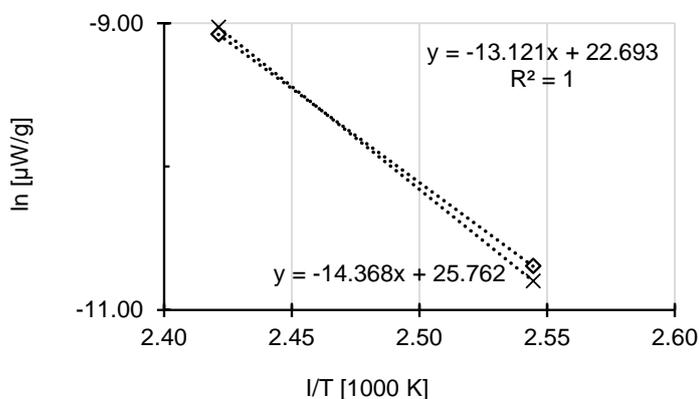
Figure 9. Activation energy for two different degree of conversion, 3 and 3.4 J/g at two different temperatures 120 and 140 °C.
