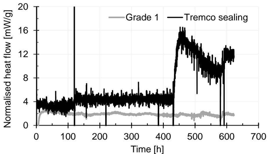
Figure 3. An Isothermal MC test at  $90 \text{ }^\circ\text{C}$  using grade 1 and Tremco sealing.
