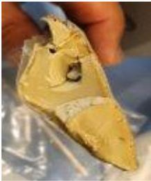
Figure 5. A cross section of Tremco sealing
