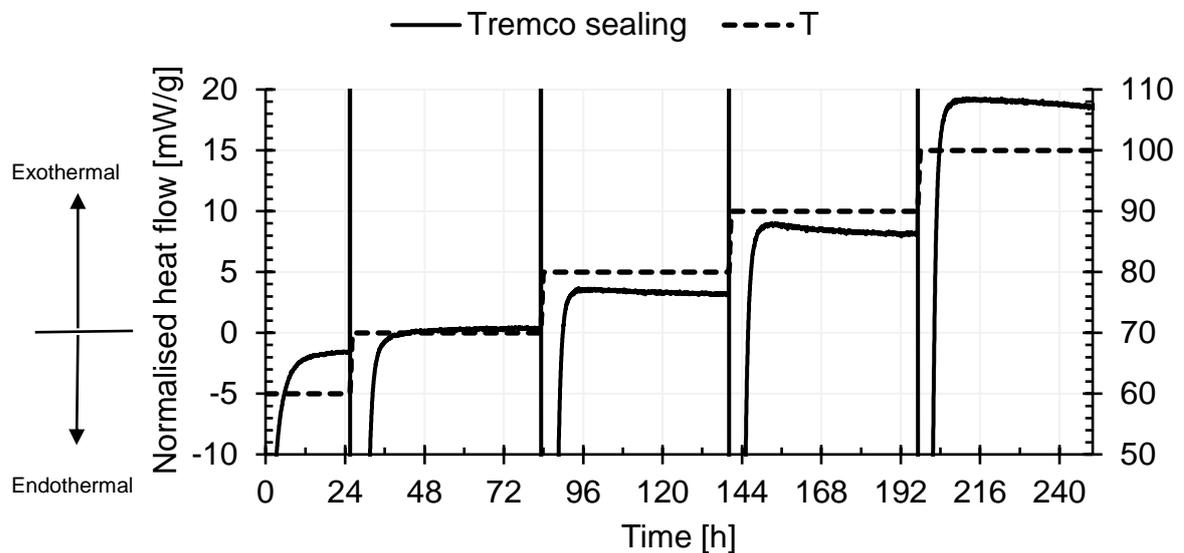
Figure 7. Normalised heat flow from a quasi-isothermal MC test at 60, 70, 80, 90 and 100 °C using tremco sealing.
