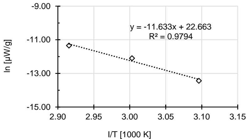
Figure 10. Arrhenius plot for commercial or grade 3 material.
