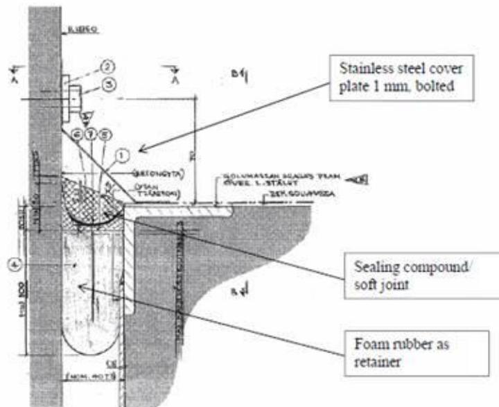
Figure 2. Tremco sealing location used in NPP
