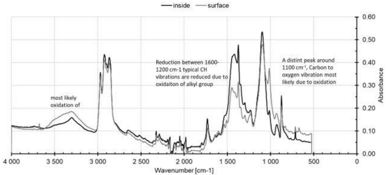
Figure 8. FTIR analysis of tremco sealing from inside and oxidised surface.
