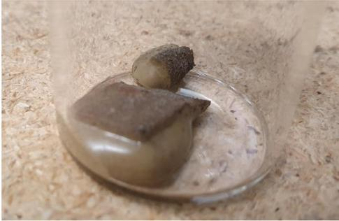
Figure 4. Tremco sealing after MC test at 90 °C.
