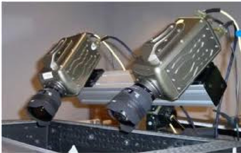
Figure 6—3 Cameras used to capture strains in the concrete, Hohmann et al. (2012).
