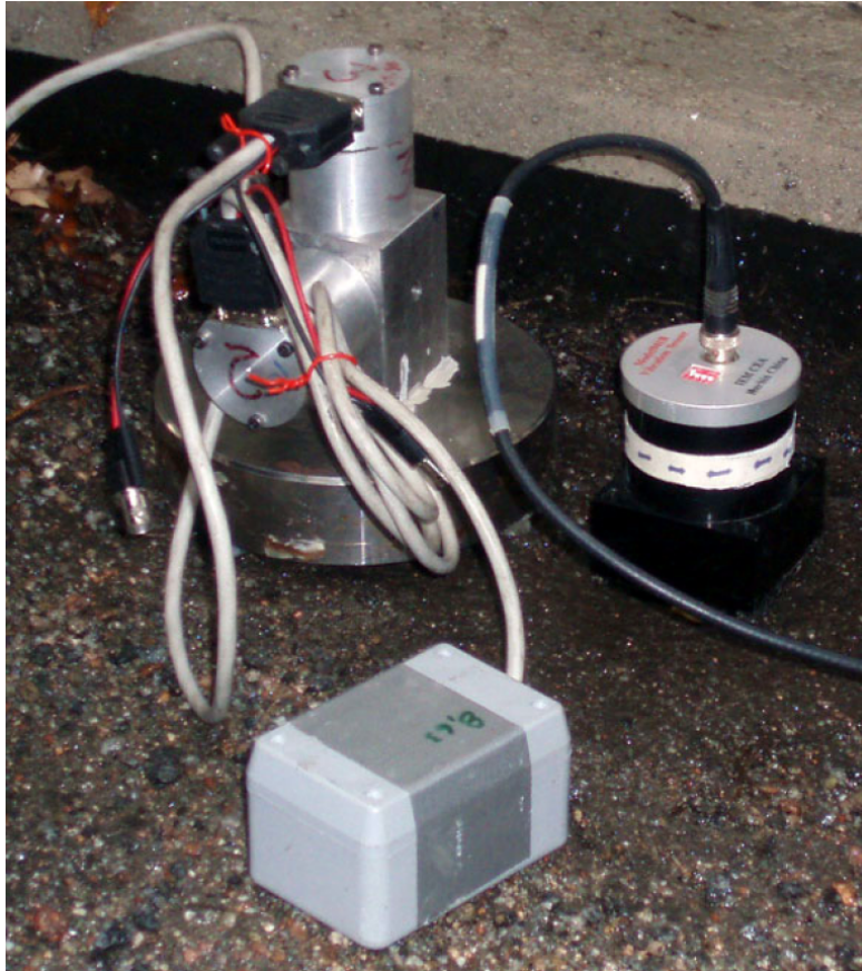
Figure 6—1 A MEMS gauge placed on the walkway of a concrete bridge, KTH (2007).
