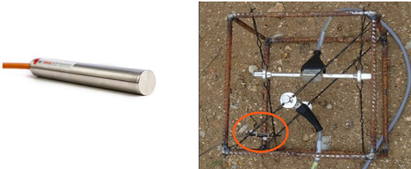
Figure 5—2 To the left, a temperature sensor for use in water and concrete, Geosense (2021). To the right, temperature sensor in a rebar cage to be cast into concrete, Oukhemanou (2016).
